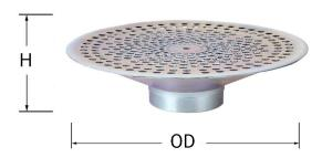
Round Hole Bottom suction strainers are used on the suction end of a suction hose to help prevent debris from being sucked into your pump. This is a critical component that helps protect your suction pump from damage or clogging. It has a female NPSM thread which connects to the male NPT on your suction hose.
