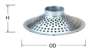
Round Hole Top suction strainers are used on the suction end of a suction hose to help prevent debris from being sucked into your pump. This is a critical component that helps protect your suction pump from damage or clogging. It has a female NPSM thread which connects to the male NPT on your suction hose.
